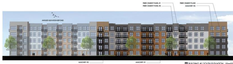
BUILDING #1 SOUTH ELEVATION
